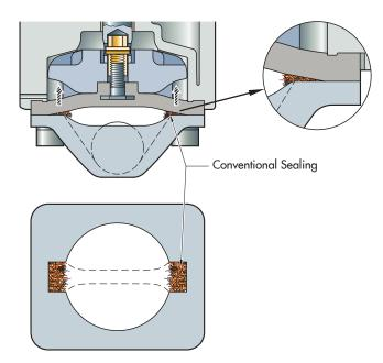
To achieve the highest level of sterility, the SED CDSA-Design Series was developed by utilizing new, qualified, and tested diaphragm valve technology. This unique design of the actuator reduces or eliminates product entrapment at the point beyond the radius of the weir on the body bonnet flange.
