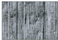
Microscopic view of mechanically polished surface with 400 grit Ra  $0.25 \, \mu m / 10 \, \mu$ -inch
