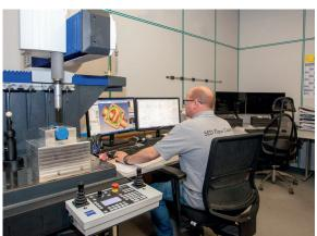
Zeiss Coordinate measuring machine (CMM)
