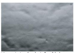
Microscopic view of mechanically polished and electro polished Ra 0,25  $\mu m$  / 10  $\mu\text{-inch}$
