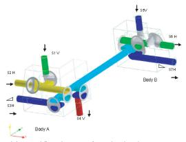
$3\mbox{D}$  modeling and flow direction of a multivalve cluster
