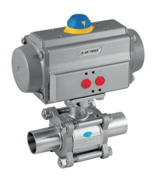
The Steriflu 342 is pneumatically operated with a piston actuator alternatively single or double acting. The pneumatic actuator has an extruded aluminium housing with internal and external Alodur special hard anodization for corrosion protection.
