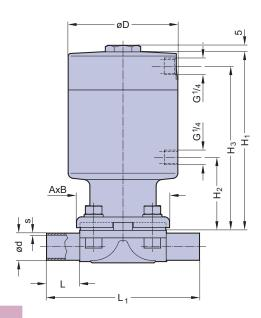
Butt weld ends MA 25 - 100 Fold out page 21
