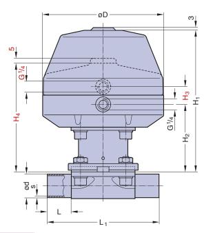
Butt weld ends MA 25 - 100 Fold out page 21
