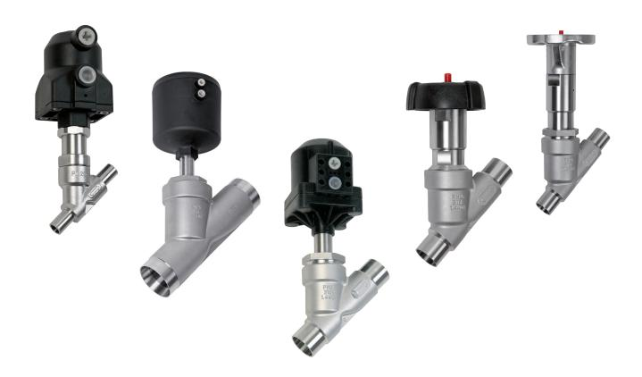
The SED Angle Seat Valve is composed of a 2/2-way angle seat valve body and a pneumatically operated piston actuator, which is mounted with a stainless steel adaption to the valve body.
