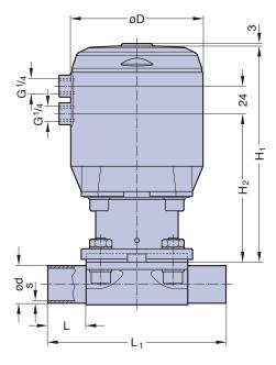
Butt weld ends MA 25 - 50 Fold out page 21
