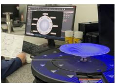
High-accuray diaphragm measurement with visual 3D coordinate measuring machine
