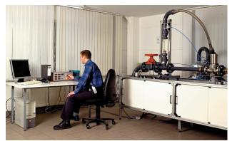
Test bench to determine and document flowrates and K<sub>V</sub> (C<sub>V</sub>) values
