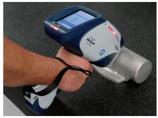
Spectrometer and XRF spectroscopy material analysis
