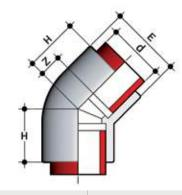
**HIF** 45° elbow for socket welding
