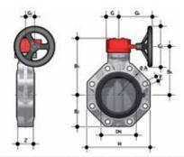
**FKOF/RM LUG ISO-DIN**Gearbox operated Butterfly valve, version Lug ISO-DIN
